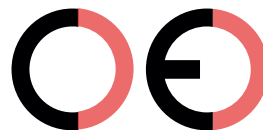
False CE Mark (too far)
